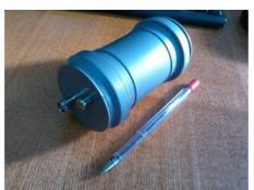
RF isolating transformer reduces the noise level and increases the S / N level. Update 8 February 2016: New PCB for mini-Whip from Singapore
