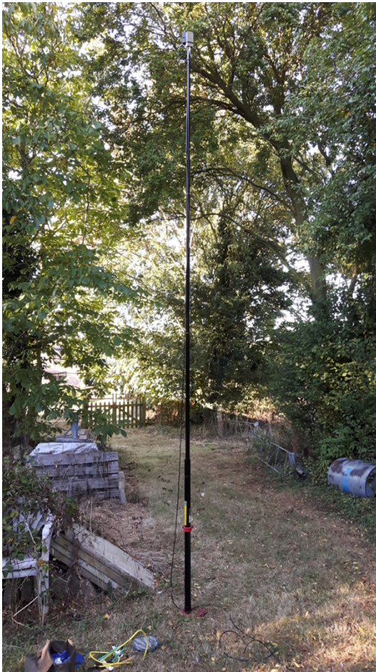
Fig 4 - Probe mounting on temporary fibreglass mast
