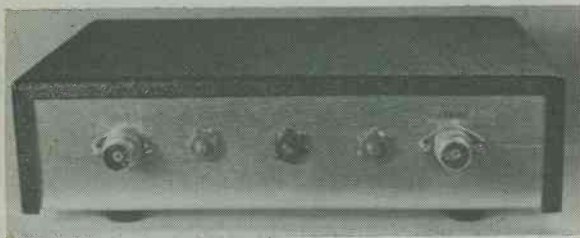
The rear of the preselector, showing the two coaxial sockets and the three plastic coil securing nuts
