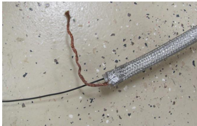
Figure 13 -- coax end with a braided wire soldered to the loop braid. Note the fish wire coming out the end.
