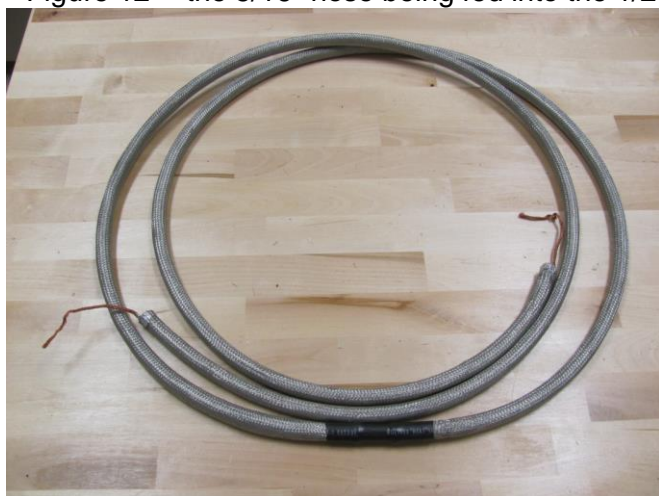
Figure 12 -- the 5/16" hose being fed into the 1/2" hose
