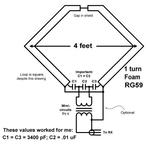
Tune C1/C3 until impedance at output connector is resistive at 1830. Then tune C2 to get 50 or 75 ohms at the output connector. Increasing C2 lowers impedance. These is some interaction, requiring an iterative method.
