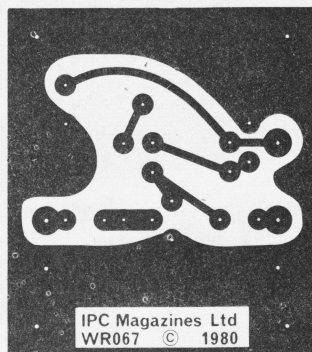
Fig. 2: Copper pattern and component layout, shown full size
