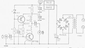
This simple aerial amplifier can be used to boost the level of weak FM signals. It has a gain of 22 dB, and the extremely low noise figure of 1.6 dB, so that it will not unduly degrade the signal-to-noise ratio.
