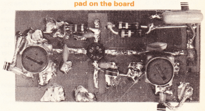
The alternative pre-amp design using a BF961 transistor and Toko coil formers with fixed tuning capacitors
