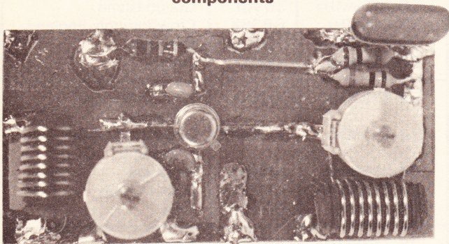
The first prototype showing the coil construction and the mounting of the metal canned transistor
